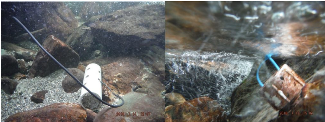
Examples of cabled temperature sensors (left) and epoxied temperature sensors (right)
